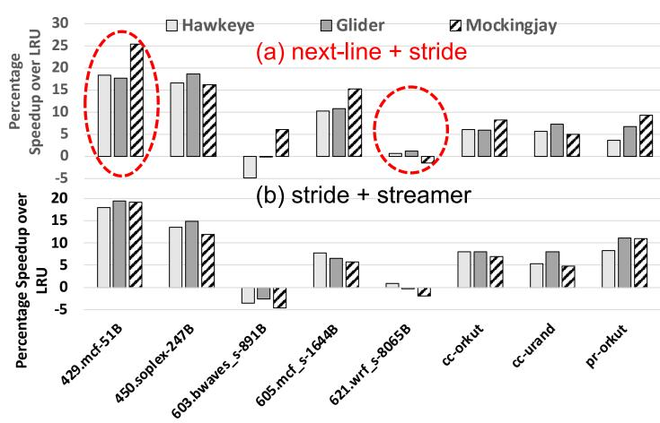
Comparing speedup over LRU on a 4-core system between: (a) using next-line prefetcher at L1 and stride prefetcher at L2, and (b) using stride prefetcher at L1 and streamer prefetcher at L2.
